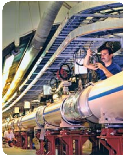
The RHIC's 2.4-mile-long concentric rings are made up of 1,740 superconducting magnets mounted end to end.
